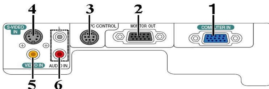
1. COMPUTER IN/Component Input Connector (Mini D-Sub 15 pin)
